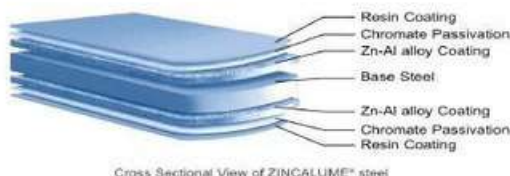
Cross-Sectional View of ZINCALUME® steel
